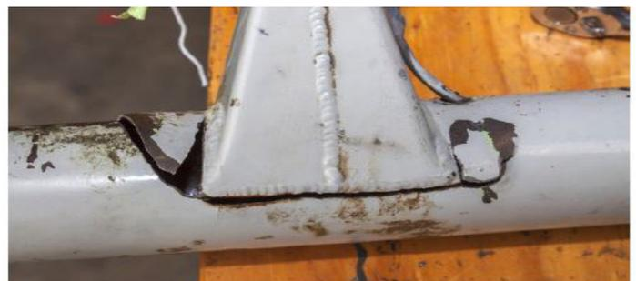
Elevator Torque Tube P/N 242646 (Item 14) – Fractured area.
