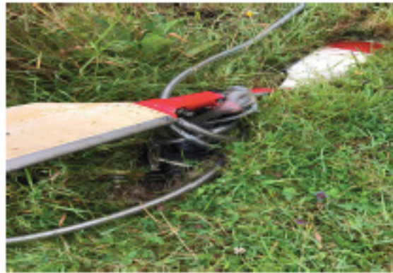
Image of the tail rotor and entangled line.
